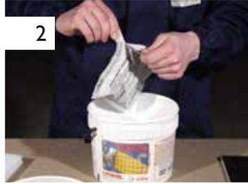
2 In the pack is the catalyst (component B). Cut the angle of the catalyst envelope.
